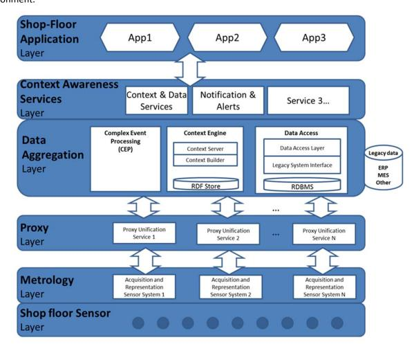
The framework is based upon a five layered architecture and each layer contributes to increasing visibility and context-awareness in a manufacturing environment by gradually enabling the easy sharing of various context information and sensor data, so that they can be used to complement each other and cover a factory-wide application environment.
